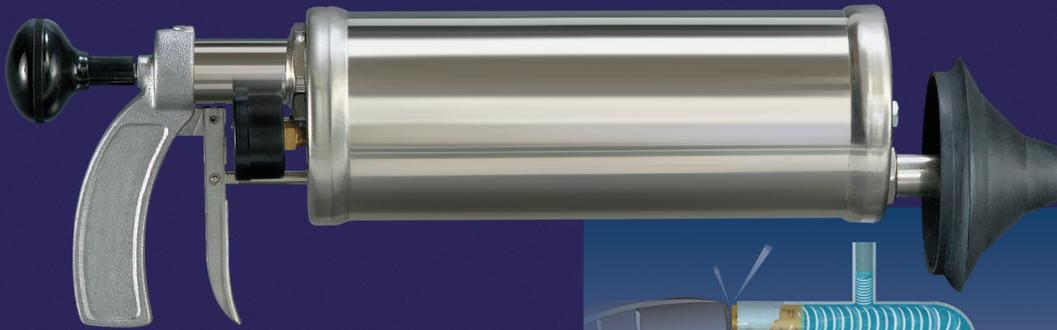
The Kinetic Water Ram uses a burst of compressed air, which strikes the column of water in a clogged pipe. The resulting shock wave, called Kinetic Energy, hits the stoppage at a speed of approximately 4,700 feet per second, quickly clearing the blockage and flushing waste particles away.
