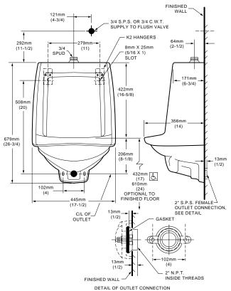
NOTES: FLUSH VALVE NOT INCLUDED AND MUST BE ORDERED SEPARATELY. PROVIDE SUITABLE REINFORCEMENT FOR ALL WALL SUPPORTS. IMPORTANT: Dimensions of fixtures are nominal and may vary within the range of tolerances established by ANSI Standard A112.19.2.
