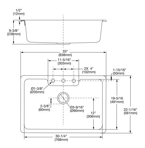
**NOTES:**\* DIMENSIONS SHOWN FOR LOCATION OF SUPPLIES AND "P" TRAP ARE SUGGESTED. FITTINGS NOT INCLUDED WITH FIXTURE AND MUST BE ORDERED SEPARATELY. SEALING COMPOUND SUPPLIED BY OTHERS.
