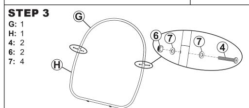
TIP: Install the bolt head on the outside of the frame, as shown.
