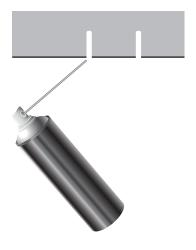
Clean loose debris from the pilot holes using a blower, canned air or a vacuum.
