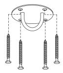
If installing into wood, position the round eye pad over the pilot holes and drive the screws into the pilot holes.
