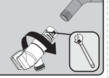
Verify that rubber sealing washer is present in hose coupling. Thread one end of hose to the outlet port of Bracket. Hand tighten.
