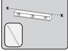
Align Mounting Plate over center point marked in previous step. Mounting Plate should be vertical as shown below. Mark Mounting Screw locations onto the wall surface. Remove items after marking mounting locations.
