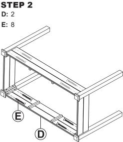
Secure 2x Side Panels (D) to the inside edges of the assembled leg/end panels using 8x M4x40mm Screws (E).
