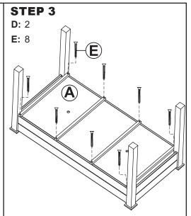
Place Bottom Panel (A) on the bottom of the assembled components, as shown.
