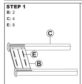
Align End Panel (B) with 2x Leg (C) and secure with 4x M4x40mm Screw (E).
