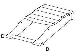
Using (2) 2" Screws fasten Cross Brace
