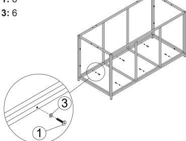
Do not fully tighten hardware until after step 5 is complete.
