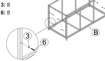
Do not fully tighten hardware until after step 5 is complete.
