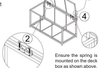
Do not fully tighten hardware until after step 5 is complete.
