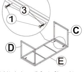
Do not fully tighten hardware until after step 5 is complete.
