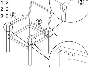
Ensure the front of each armrest is aligned with the leg and secure using Bolt (1).
