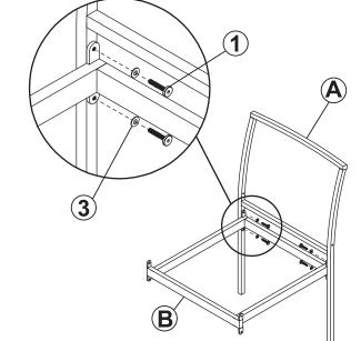
Connect Seat (B) to Back Panel (A) using Bolts (1) and Washers (3).
