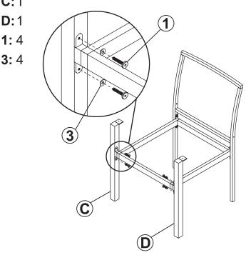
Connect Legs (C, D) to the seat using Bolts (1) and Washers (3).
