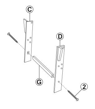
Do not fully tighten hardware until Step 6 is complete.
