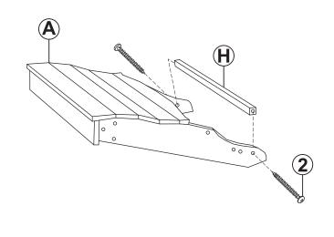
Do not fully tighten hardware until Step 6 is complete.
