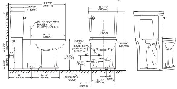
**IMPORTANT:** Water supply on the wall is required at 3" (76 or 229mm) from centerline of the toilet (see rough-in). First suggested position is hidden behind the toilet. The geometry of the toilet gives space for this installation. The second suggested position is next to the toilet. Between these two positions, the space for the supply between wall and toilet is limited to 3-1/2" (89mm). In this case, check your supply and hose dimensions.
