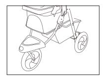
4. Attach the foot board by positioning it to the bottom and tightening screws.
