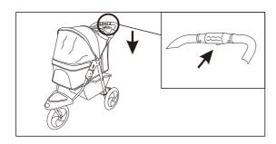
9. To fold the stroller: unzip the canopy window first, then press the folding button to fold the stroller and fasten the folding hook.
