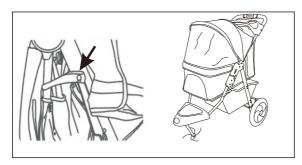
1. To open the stroller: release the folding hook as shown in the picture, lift the handlebar, unfold the stroller and make sure both joints are locked.
