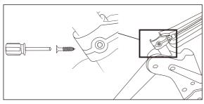
2. To install the canopy: Attach the plastic buckle on the pole and use the screws to secure it in place.
