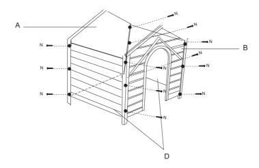
1) Secure all 4 walls (parts A,B,D) with 12 screws (part N) as shown above.
