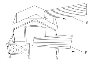
3) Place Part F on the porch for the floor, as shown above. Part E will be placed inside the house for the dog house flooring.
