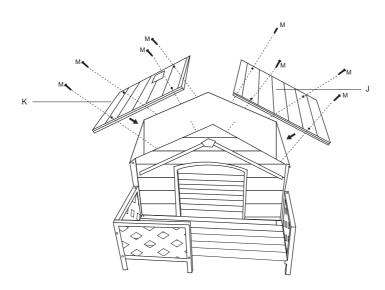
4) To assemble the roof, place part K on the left and part J on the right. Secure the roof with 8 screws (part M).
