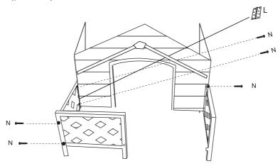
2) Assemble the fence with 3 screws (Part N). Use 2 screws (Part N) to place Part L on the left side of the fence.
