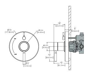
VALVE MOUNTING IS SHOWN FOR REFERENCE ONLY. VALVE IS NOT INCLUDED WITH CPT-1400-P / CPT-1400-KN
