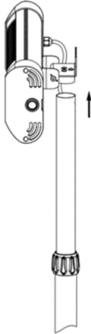
Step 4: Screw the handle through the top tube support cap into the top tube.
