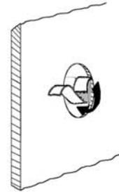
Wrap Plumbers Tape around the pipe threads. It may be necessary to attach a pipe nipple (not included) to the supply line for your installation.
