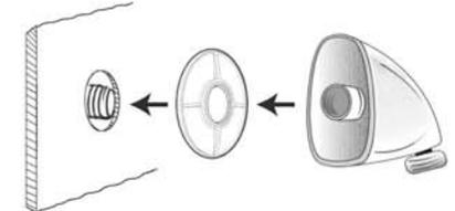
Secure the gasket around the pipe to assist in making a good seal between the supply elbow and shower wall. Fit the threads on the back of the supply elbow to the threads on the pipe and hand tighten until snug.
