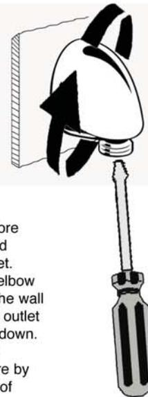
To fully tighten the supply elbow, insert a #2 Phillips screwdriver into the outlet on the supply elbow, making sure the screwdriver reaches all the way into the supply elbow before tightening to avoid breaking the outlet. Tighten until the elbow is firmly against the wall and the threaded outlet is facing straight down. Make sure not to over-tighten where by the gasket is out of round.
