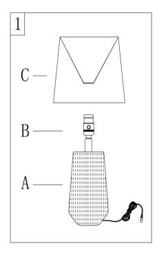
Step1 Place shade(C) onto the Socket(B).
