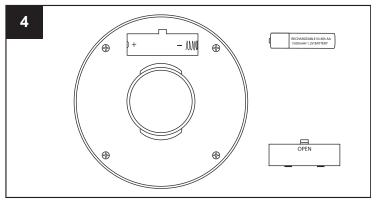
Remove the old battery. Paying attention to the positive and negative terminals, insert the new battery.
