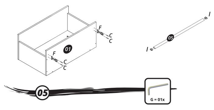
Pass the part (05) through the hardware (F) and use the hardware (G) to tight the screw as shown on detail.
