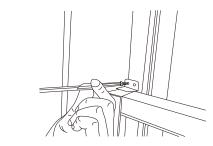
**Fig.9**D.Cut Window sash seal foam and insert it in the space between the upper and lower sashes (Fig.10).
