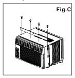
NOTE: For safety reasons, all four(4) screws MUST be securely fastened.
