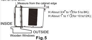
**NOTE:** Check that air conditioner is tilted back about H (Fig.5)(tilted about 3° to 4° downward to the outside). After proper installation, condensate should not drain from the overflow drain hole during normal use, correct the slope otherwise.
