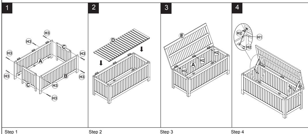
Attach font panel (B) and back panel (A) to leg frame (C) by using screw (H3), tighten with allen (H4)
