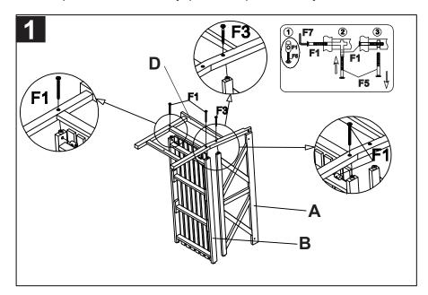
Step1: attach the left side (D) to the seat (B), back (A), bottom (C) as shown on the picture. Using the Allen bolt (F1), the Allen screw (F3) and tighten with the Allen key (F7). Make sure you don't tighten too tight and you will do at the end.
