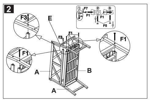
Step 2: repeat with the right side (E) as step 1 as shown on the picture. At last tighten all bolts and screws.
