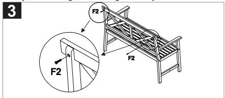
Step 3: Use the Allen bolt S (F2) to fix the back (A) as shown on the picture by using the Allen key (F7).
