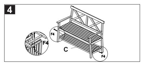
Step 4: put the bottom (C) using the Allen nut (F4) as shown on the picture. Tighten the Allen nut (F4) by using the Allen key (F7) and wrench (F6).
