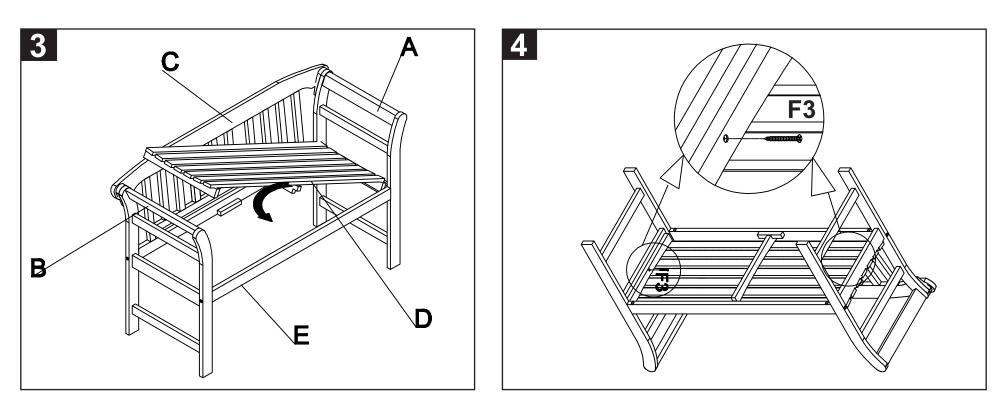
Step 3: put the seat (D) inside the bench as shown on the picture.
