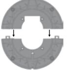
2. Assemble the base to the bottom of the tower. There is an alignment pin (A) located on the bottom of the tower and an alignment recess (B) located on the base. An arrow on bottom of base indicates alignment recess location. To ensure correct assembly, position base onto bottom of tower with (A) and (B) aligned. Take care that power cord is routed through hole on base before moving to next step in assembly.
