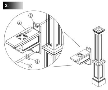
Secure the paper holder arm (part 2) to the decorative post (part1) using two 3" lag bolts (part 4) for the top and two 3" screws (part 5) in the bottom. Plastic snap caps (part 6) are provided to cover the screw heads.
