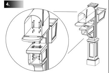
Pre-drill 4 holes with a 3/8" drill bit through the mailbox and paper holder arm as shown above. Using a nut, bolt, and washer combination secure the mailbox to the arm and tighten. 2" bolts are recommended (mailbox and mailbox mounting hardware not included). Heavier boxes can be reinforced by securing 2 screws through the back of the mailbox directly into the post.
