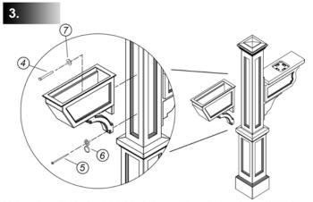
Using the pilot holes provided, fasten the planter (part 3) to the post as shown. Use one 3" lag bolt (part 4) and washer (part 7) in the top part of the arm and one 3" screw (part 5) for the bottom. A snap cap (part 6) is provided to cover the screw head.
