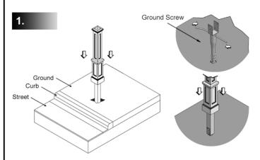
Dig a 24" deep hole in the desired location and insert a 4x4 wood post. Leave 48" exposed above ground. Fill the hole with pre-mix concrete (not included) and level the wood post. Once the concrete has cured, slide the decorative post (part 1) over the wood 4x4 ensuring that the base sits flush with the ground.
