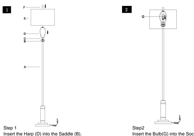
Insert the Bulb(G) into the Socket(C).
