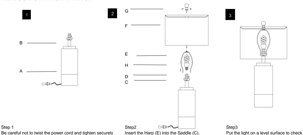
Put the shade(F) on the Harp(E),then tighten the Finial (G)into the Harp (E) Insert the bulb(H) into the socket(D).
