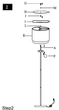
Insert the Bulb(F) into the socket.
