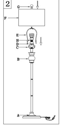
Insert the Harp (E) into the Saddle (C).
