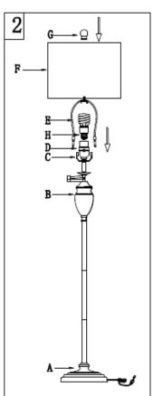
Step2 Insert the Harp (E) into the Saddle (C). Put the shade(F) on the Harp(E), then tighten the Finial (G) into the Harp (E) Insert the bulb(H) into the socket(D).
