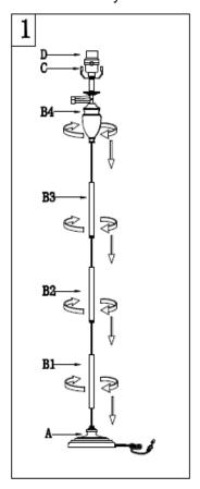
Step 1 Screw the Lamp body (B4) onto the Lamp body (B3) Screw the Lamp body (B3) onto the Lamp body (B2) Screw the Lamp body (B2) onto the Lamp body (B1) Screw the Lamp body (B1) onto the Lamp base (A) Be careful not to twist the power cord and tighten securely
