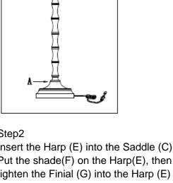
Step2 Insert the Harp (E) into the Saddle (C). Put the shade(F) on the Harp(E), then tighten the Finial (G) into the Harp (E) Insert the bulb(H) into the socket(D).
