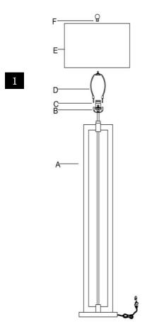
Step 1 Insert the Harp (D) into the Saddle (B). Put the Shade(E) on the Harp(D),then tighten the Finial (F)into the Harp (D)
