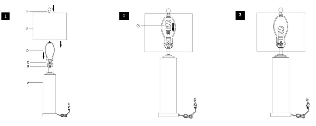
Step 1 Insert the Harp (D) into the Saddle (B). Put the Shade(E) on the Harp(D),then tighten the Finial (F)into the Harp (D)
