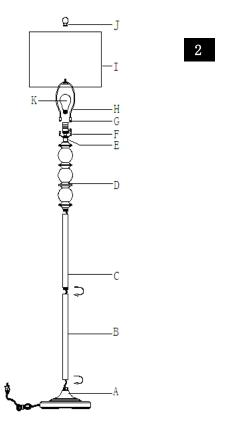
Step2 Insert the Harp (H) into the Saddle (F). Put the shade(I) on the Harp(H),then tighten the Finial (J)into the Harp (H)
