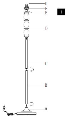
Step 1 Make sure all parts could be aligned before assemble Do not rotate lamp body too hard avoid base screm broken Pull cord through lamp base(A) to tighten stem connections, make sure the screw nut at the bottom of the lamp is tightened. Insert the bulb(K) into the socket(G). Fasten tube(B) onto base(A).Fasten tube(C) onto tube(B)
