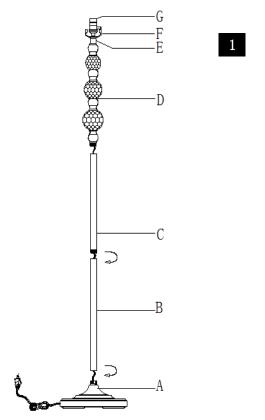
Step 1 Make sure all parts could be aligned before assemble Do not rotate lamp body too hard avoid base screm broken Pull cord through lamp base(A) to tighten stem connections, make sure the screw nut at the bottom of the lamp is tightened. Insert the bulb(K) into the socket(G). Fasten tube(B) onto base(A).Fasten tube(C) onto tube(B)
