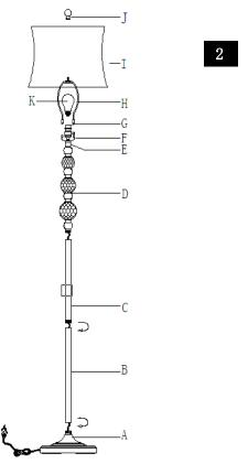
Step2 Insert the Harp (H) into the Saddle (F). Put the shade(I) on the Harp(H),then tighten the Finial (J)into the Harp (H)
