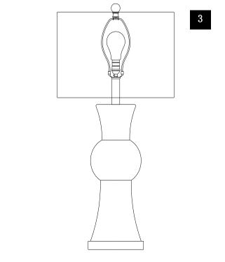
Step 1 Screw the Neck (B) onto the Lamp base (A) Be careful not to twist the power cord and tighten securely
