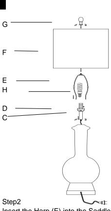
Insert the Harp (E) into the Saddle (C). Put the shade(F) on the Harp(E),then tighten the Finial (G)into the Harp (E) Insert the bulb(H) into the socket(D).
