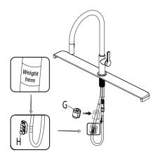
Install the weight clip (H) at the point of the hose marking "weight here". Insert the weight (G) onto the weight clip (H) by sliding it down onto the weight clip (H).
