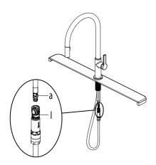
Push the quick connector (I) firmly upward and attach it to the receiving block (a). Pull down moderately to ensure the connection has been made.
