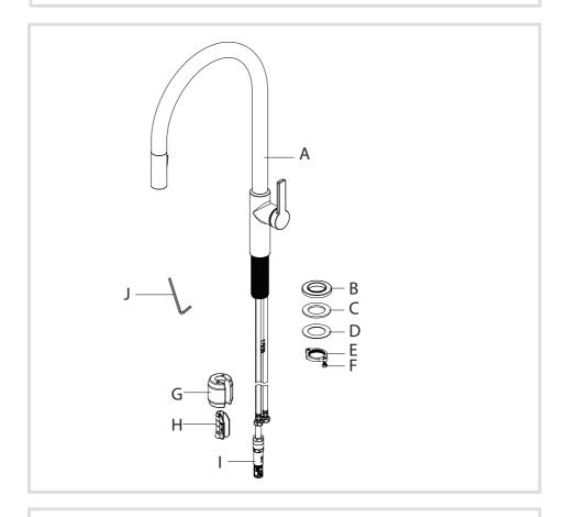
A. Faucet BodyF. ScrewsB. FlangeG. WeightC. Rubber WasherH. Weight ClipD. Metal WasherI. Quick ConnectorE. Mounting NutJ. Hex Wrench
