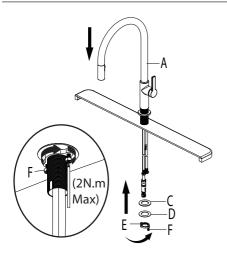
Shut off the water supply. Place faucet (A) through the hole in countertop. Secure the faucet (A) to the countertop using the rubber washer (C), metal washer (D) and mounting nut (E) provided. Tighten screws (F).
