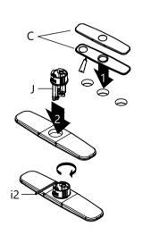
Place a bead of clear silicone sealant (not included) around the edge of the putty plate (C). Secure deck & putty plate (C) on sink or countertop. Insert base (J) into hole of deck & putty plate (C) with "FR1NT" facing forward. Tighten screws on base (J) with 4mm hex wrench (i2) until base is secure on deck & putty plate (C).
