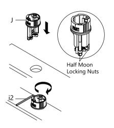
Insert base (J) into sink or countertop with "FR†NT" facing forward. Tighten screws on base (J) with 4mm hex wrench (i2) until base is secure on sink or countertop.
