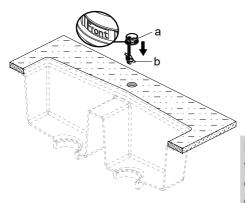
Shut off the water supply. Remove the old faucet. Clean the mounting surface. Check for the proper thickness of the sink. Insert the base (a) into sink.
