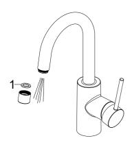
After installing faucet, remove aerator. Turn water on for 30 seconds to remove any debris. Reassemble aerator. Do not lose the gasket (1) in the aerator.
