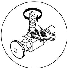
Connect hot and cold waterlines (7) to the angle stops. Tighten with a wrench until snug. Turn on hot and cold angle stops and check for leaks.
