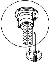
Adjust direction of faucet body (5). Tighten mounting nut (6C) until snug. Tighten mounting screws (6D) to nut with a Phillips head screwdriver until snug.
