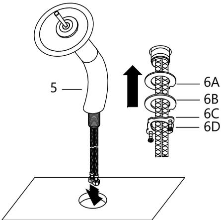
Insert faucet body (1) into the hole on the countertop. Attach rubber washer (6A), metal washer (6B), mounting nut (6C), and mounting screws (6D) from underneath the sink.
