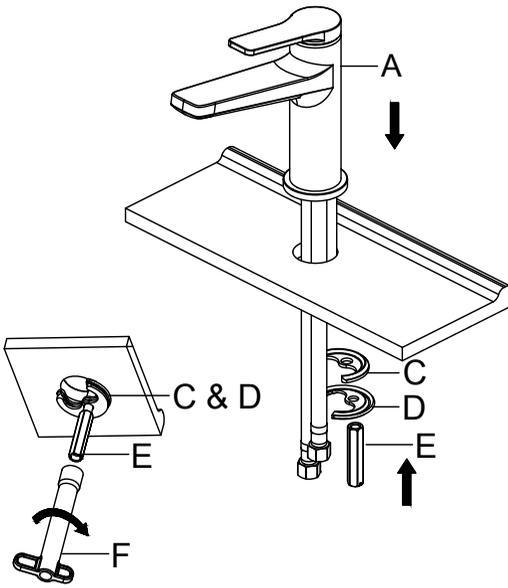
Place the faucet (A) through the mounting holes in the sink until the faucet (A) sits on top of the sink. Secure the faucet (A) to the sink using the rubber (C) and metal washers (D) and lock nut (E) provided. Ensure the washers (C&D) and waterlines have no interference.
