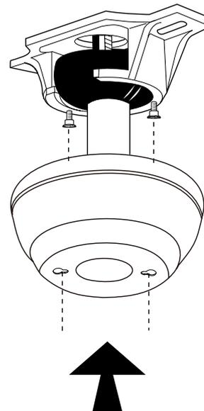
1. Notice the half ball on the end of the support rod is grooved down one side. This key way fits over the small keyway pin on the inside of the mounting bracket and keeps the ceiling fan from spinning on the mounting bracket.
