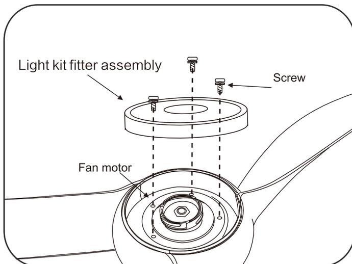
1. As shown in the picture, remove the 3 screws on the motor, install the lamp plate on the motor, and lock the screws.
