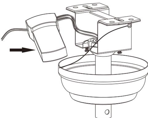
1. Carefully push the canopy to the bottom of the mounting bracket, make two sliding holes aligned to the two prominent screws on the mounting bracket, and then turn clockwise until tight.
