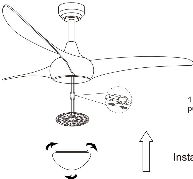
1. Connect the light kit with motor, put the light kit in the light kit fitter.
