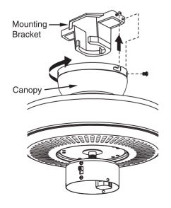
Slide the canopy up into place over the ceiling mounting bracket. Loosen up the canopy screws on the side of the canopy screws. Press the canopy against the mounting bracket and turn it clockwise. Tighten screws on the J Slots and install the two screws in the remaining holes.
