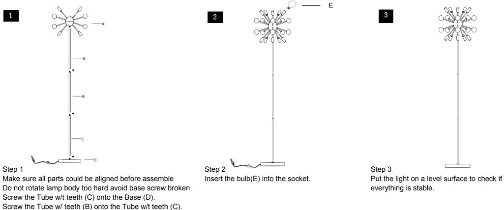
Screw the Tube w/ teeth (B) onto the Tube w/ teeth (B). Screw the Socket Assembly (A) onto the Tube w/ teeth (B)
