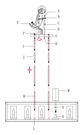
PLEASE USE ON/OFF TYPE"B" BULB MAX 40-WATT OR CFL BULB MAX 13-WATT OR LED BULB MAX 9-WATT.THERE ARE 5PCS LED 4-WATT BULB IN THE BOX
