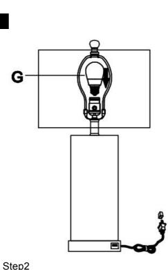
Insert the bulb( G) into the socket(C).
