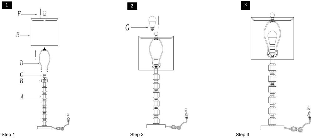
Insert the Harp (D) into the Saddle (B). Put the shade(E) on the Harp(D), then tighten the Finial (F)into the Harp (D)
